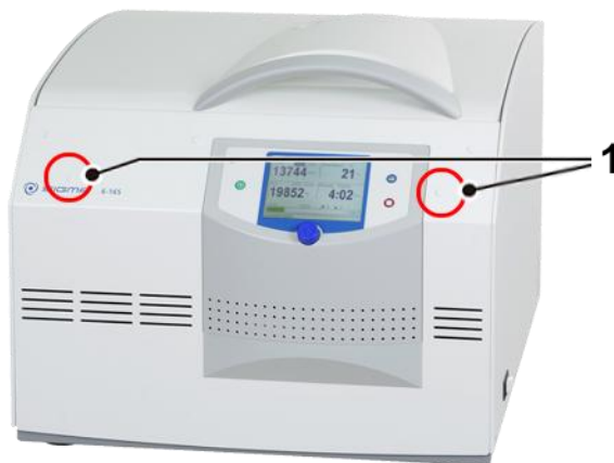
Fig. 34: Position of the openings for the emergency lid release
