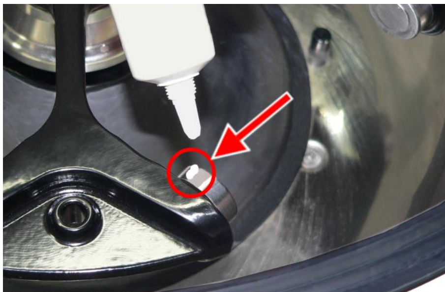
Fig. 36: Sufficient quantity of grease for one bolt
