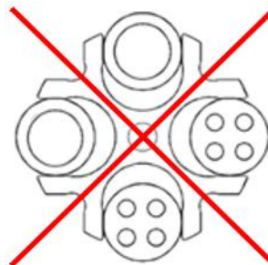
Fig. 10: Permissible and impermissible loading of a swing-out rotor with vessels of various sizes (example illustration)
