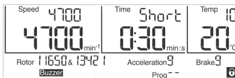
Fig. 19: Indication "Short" during a short run
