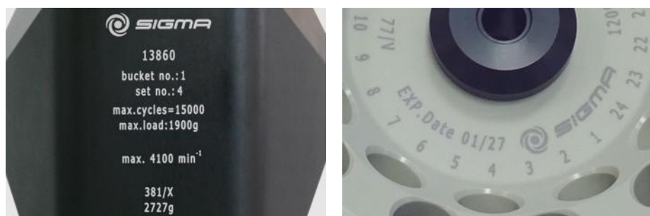
Fig. 5: Different service life – engraving on the bucket/rotor
