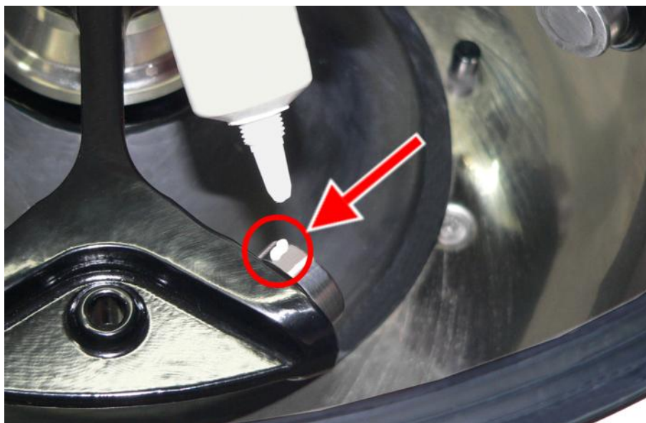
Fig. 33: Sufficient quantity of grease for one bolt
