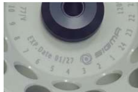
Fig. 2: Different service life – engraving on the bucket/rotor
