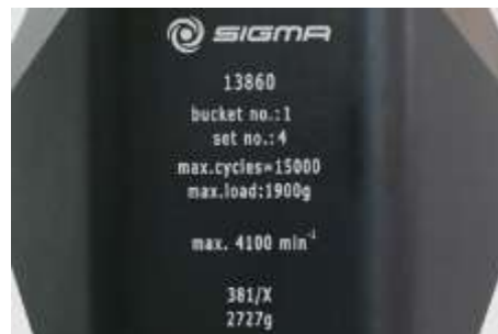
Fig. 2: Different service life – engraving on the bucket/rotor
