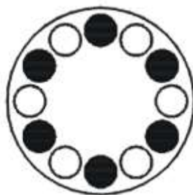
Fig. 5: Permissible and impermissible loading of an angle rotor (example illustration)
