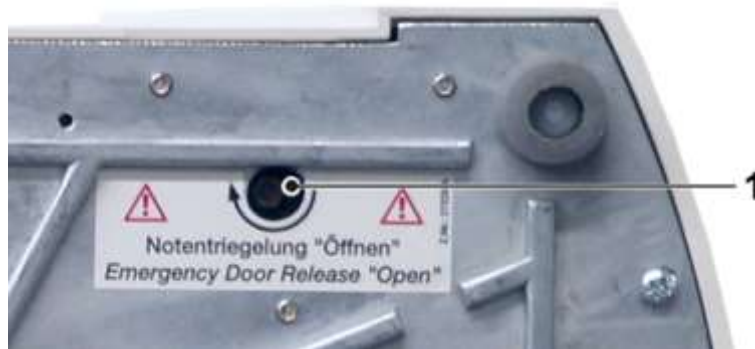
Fig. :8 Opening for the emergency lid release at the bottom of the centrifuge
