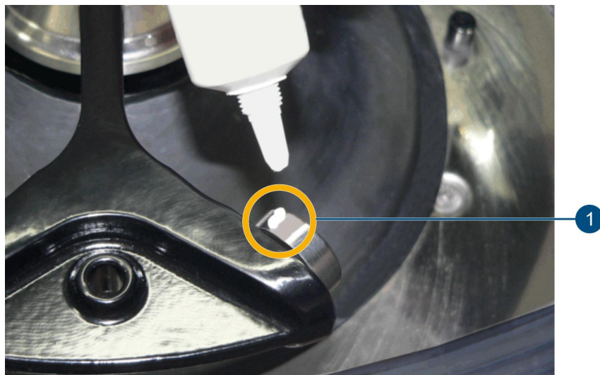
Fig. 71: Applying the grease for load-bearing bolts
